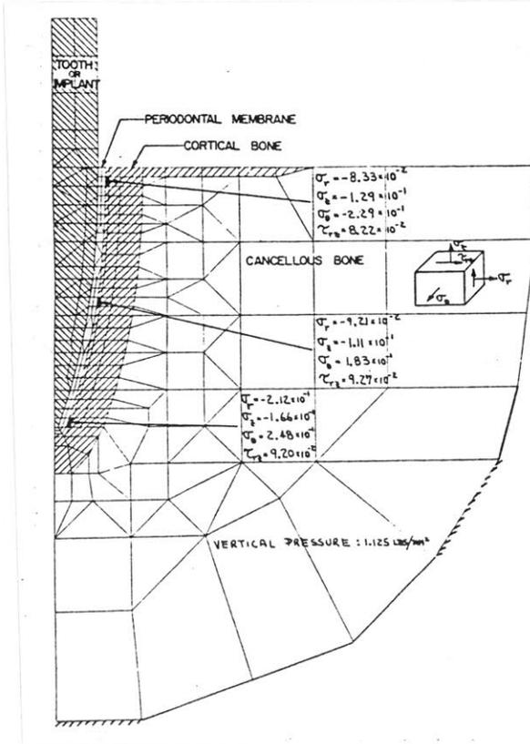
Figure 57 Finite element model of implant, periodontal membrane and the mandible, (Widera et al., 1976).
