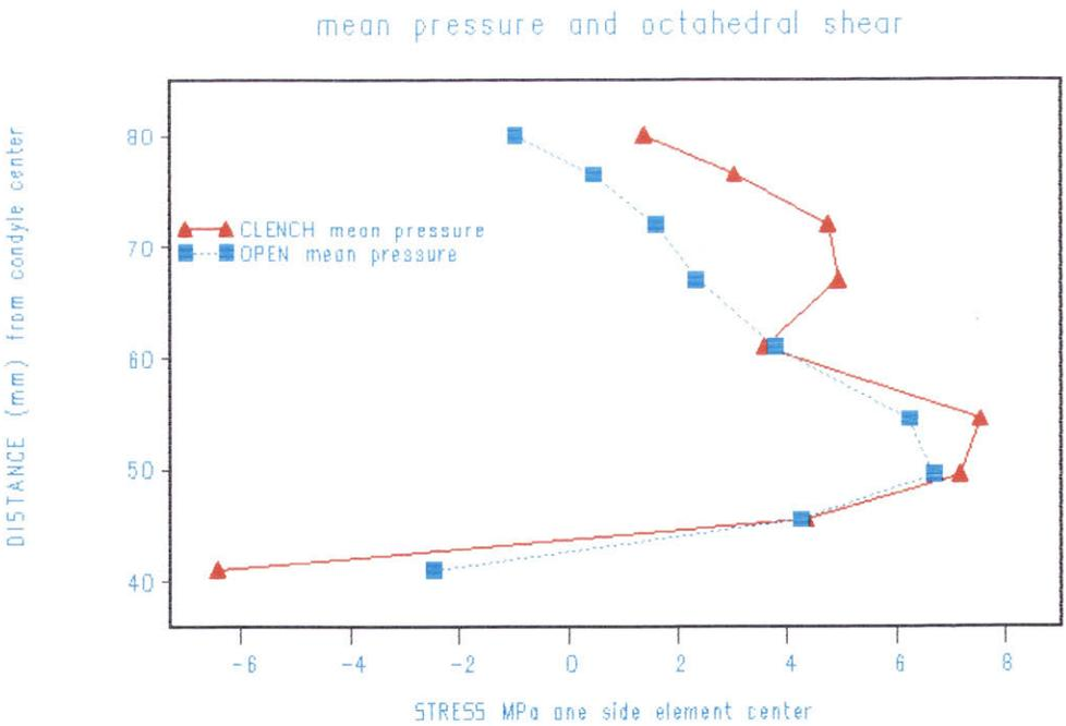
Figure 89 Comparison of mean pressure during wide open and clenching along the most protruding point on bony ridge.
