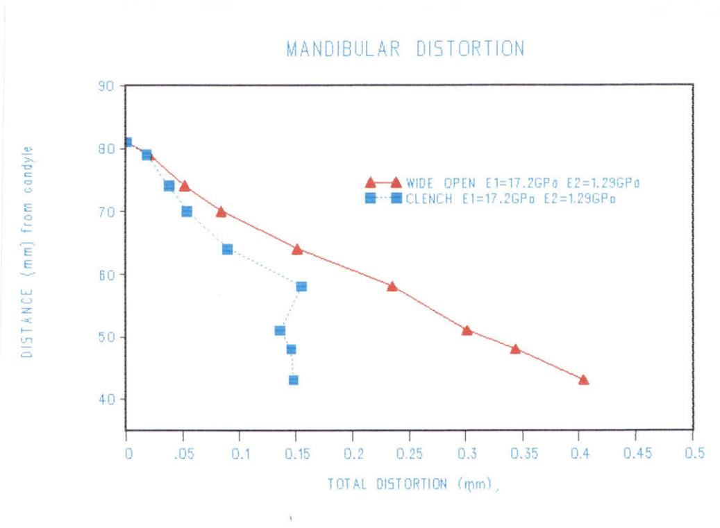
Figure 85 The distortional change of the mandible during wide opening and clenching ( $E_1 = 17.2 \text{ GPa}$ ,  $E_2 = 1.29 \text{ GPa}$ ).
