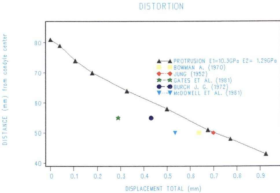
Figure 97 Comparison of the measured and the calculated distortional values during protrusion.  $E(\text{cortical}) = 10.3 \text{ GPa}$ ;  $E(\text{cancellous}) = 1.29 \text{ GPa}$ .
