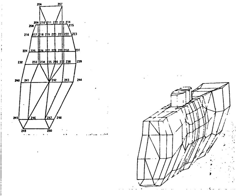
Figure 59 a) Buccal-lingual finite element grid centre selection; b) Three-dimensional finite element model (Weinstein et al., 1980).
