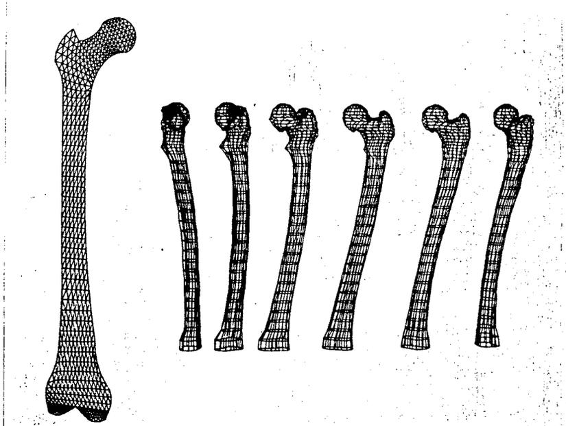
Figure 51 Element meshes of the human femur; 2-D mesh of 936 triangular 3-node elements (537 nodes)(Brekelmans et al. 1972); 3-D mesh of 1950 8-node isoparametric hexahedron elements (2532 nodes)( Rohlmann et al.,1980).
