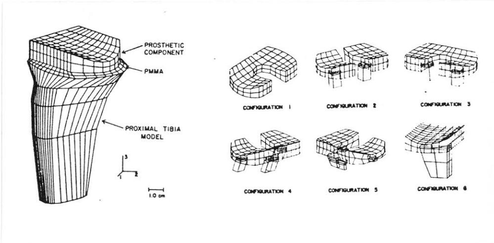
Figure 54 A 3-D FEM model of 768 eight node linear isoparametric hexahedron elements to investigate the tibial plateau fixation of total knee replacement (Lewis et al.,1982).
