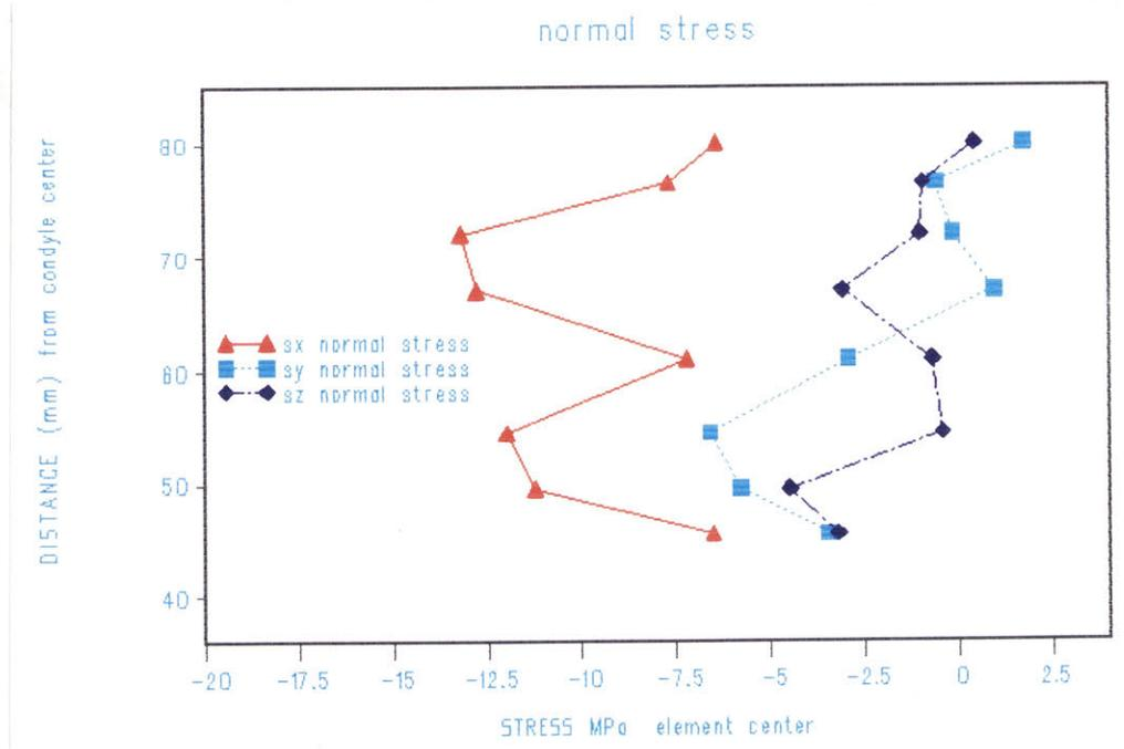
Figure 90 Normal stresses along the most protruding point on the bony ridge.
