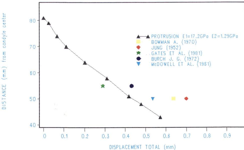
Figure 96 Comparison of the measured and the calculated distortional values during protrusion.  $E(\text{cortical}) = 17.2 \text{ GPa}$ ;  $E(\text{cancellous}) = 1.29 \text{ GPa}$ .
