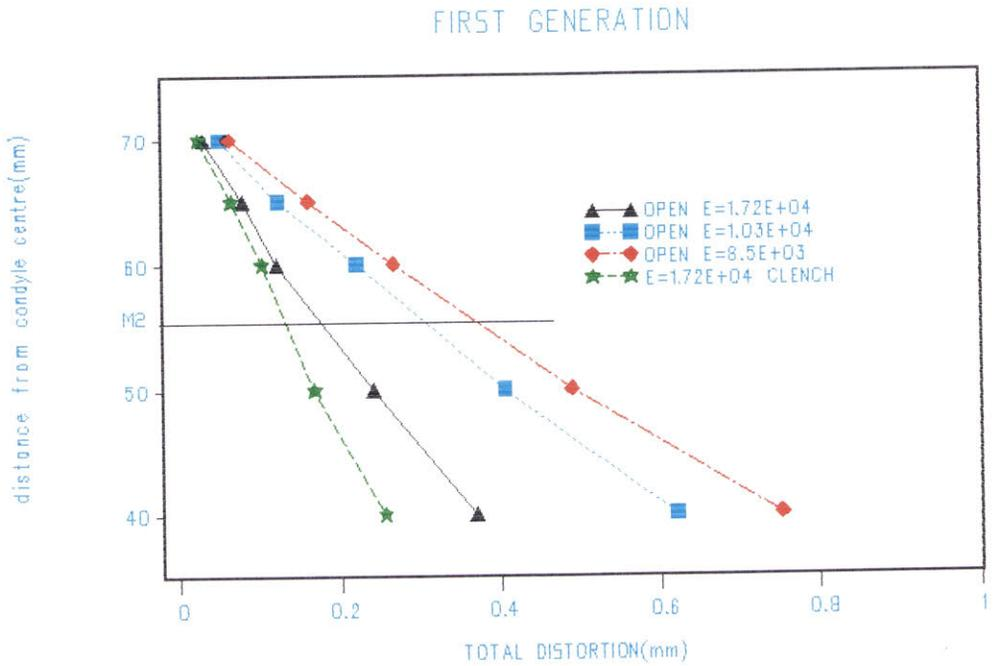
Figure 83 Distortion v.s the distance from condyle centre at various Young's modulus values under the clenching and opening conditions.
