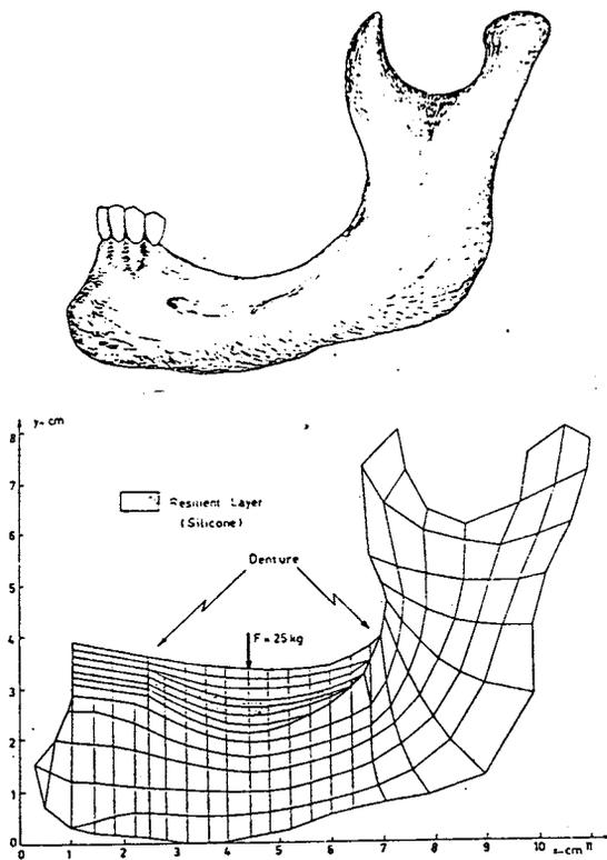
Figure 63 Finite element mesh of the mandible with a removable partial denture. (Aydinlik and Akay, 1980).
