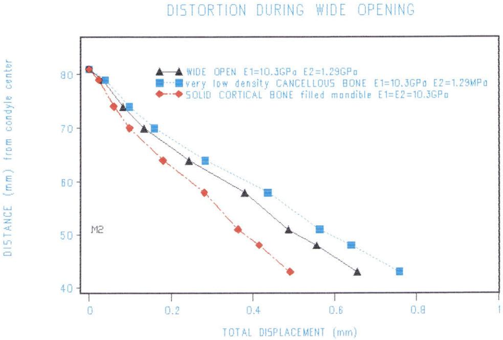
Figure 92 Comparison of hollow and solid mandibular bone, distortion values.
