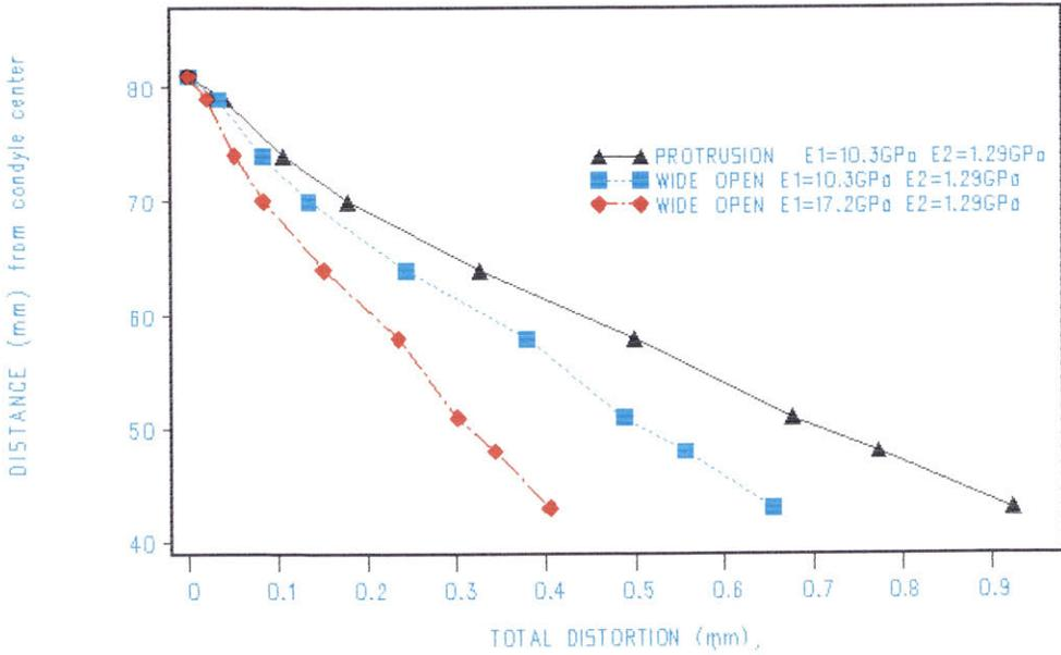
Figure 95 Comparison of distortion values of mandible during opening and protrusion.
