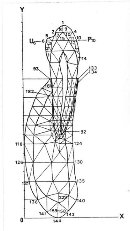
Figure 58 Finite element model of first premolar (Kitoh et al., 1977).
