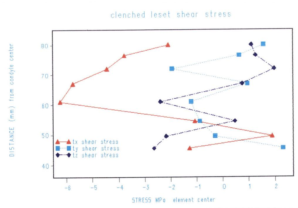
Figure 91 Shear stresses along the most protruding point on the bony ridge.
