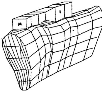
Figure 62 Representation of the three-dimensional finite element model; (M) Molar, (I) implant (Cook et al., 1982).
