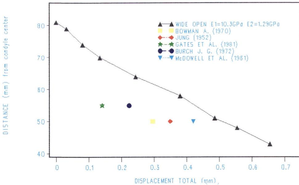
Figure 100 Various measurement values of distortion during wide opening movement.  $E(\text{cortical})= 10.3 \text{ GPa}$ ;  $E(\text{cancellous})= 1.29 \text{ GPa}$ .
