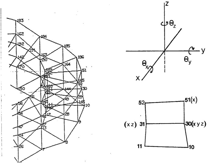
Figure 72 Finite element model of the constrained section (a), and Possible rigid body motions (b).
