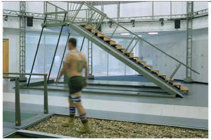
The Gait Lab is fitted with 24 motion capture cameras, mounted on a customdesigned automated truss, which use infrared light to analyze human motion across different terrains. Force plates in the floor, parallel bars and treadmills measure ground reaction forces.
