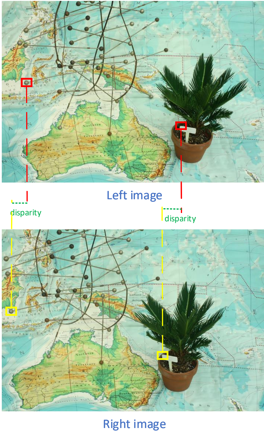
Figure 1.2: An example of disparity. The red box and red line are the pixels from the left image, and the yellow box and yellow line are the corresponding points on the right image. The disparity is shown as a green dotted line.
