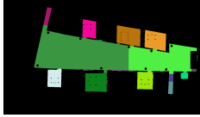
Figure 6.2: This shows the segmentation as determined by Bormann et al [2]. If one looks at the largest, centre room it is clear to see why they have achieved high precision but relatively low recall. Both segmented regions are fully contained within the ground truth and hence high precision is achieved. However, the ground truth is not even nearly contained within either segmented region and hence recall is low.
