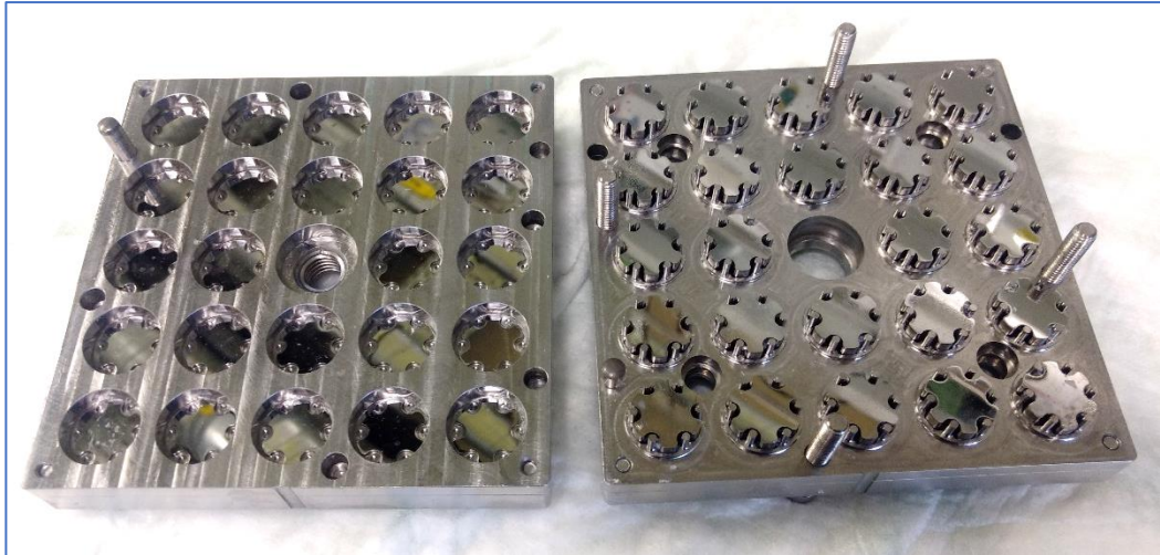
Appendix-figure 1 Aluminium casting mould for PDMS stretch chambers.
