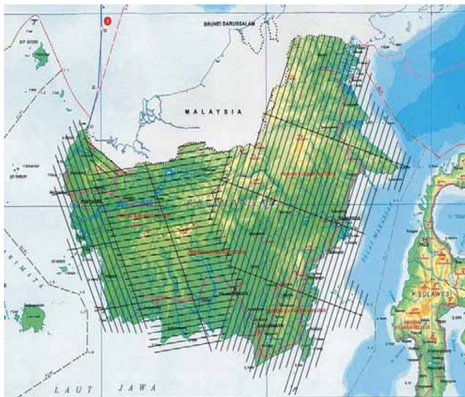
Figure 7.1 Draft survey layout for airborne gravity over Kalimantan. Total flight volume is approximately 400 hours airborne.
