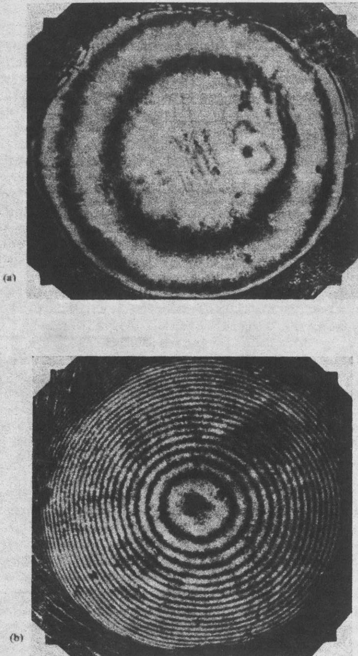
Fig. 2. Interference fringes. (a)  $R=450$  cm, (b)  $R=50$  cm.
