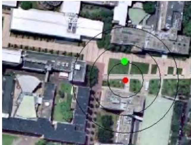
Figure 7. 15 Positioning result for the query image shown with green dot. The red dot indicates the location determined by the GPS, with the black circles show the process to enlarge the search space (1-3 times of its horizontal precision).
