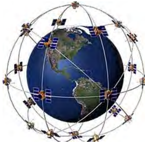
Figure 1. 1 The GPS satellite constellation (Griffin, 2011)
