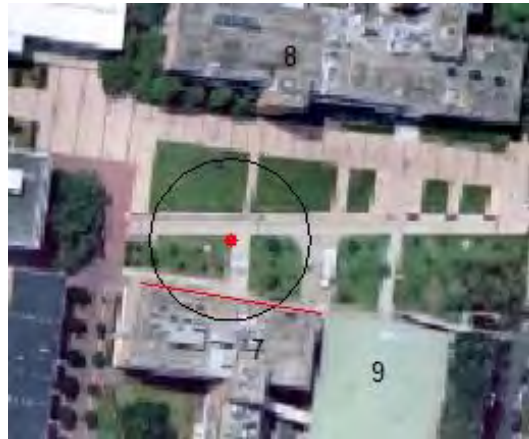
Figure 7. 3 Given a GPS position data from mobile device at P shown with red dot, a circle is drawn with 20m radius representing the search space. Line segment from building No. 7 crossed with the circle, so reference images of building No. 7 are chosen for image space
