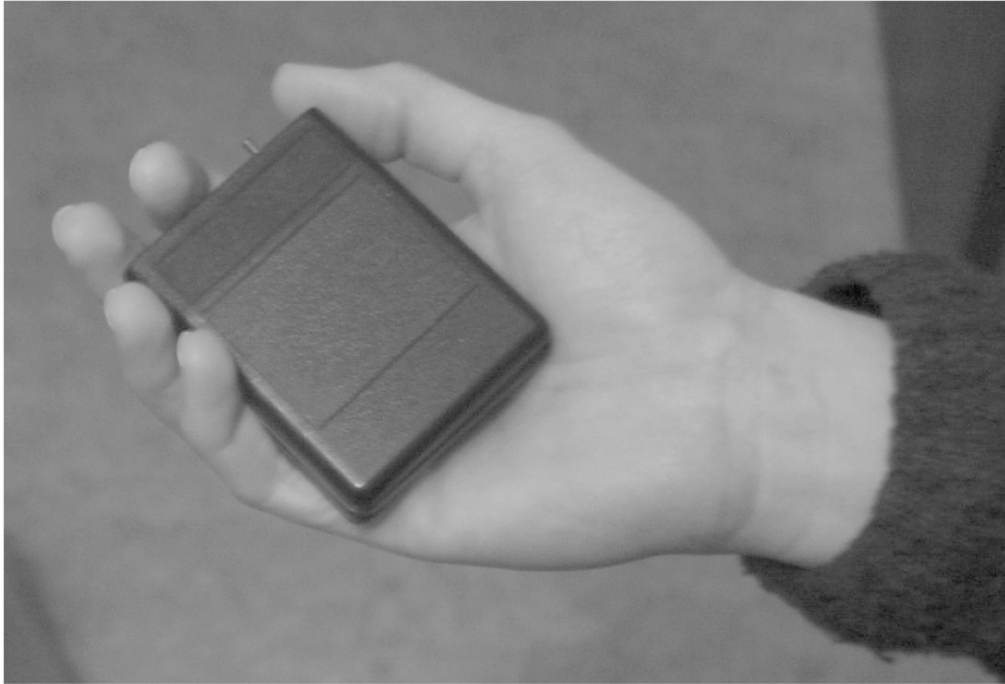
Figure 4.2: Photograph of the ambulatory monitor. The accelerometers were contained in a pager casing measuring 71 \times 50 \times 18 mm.
